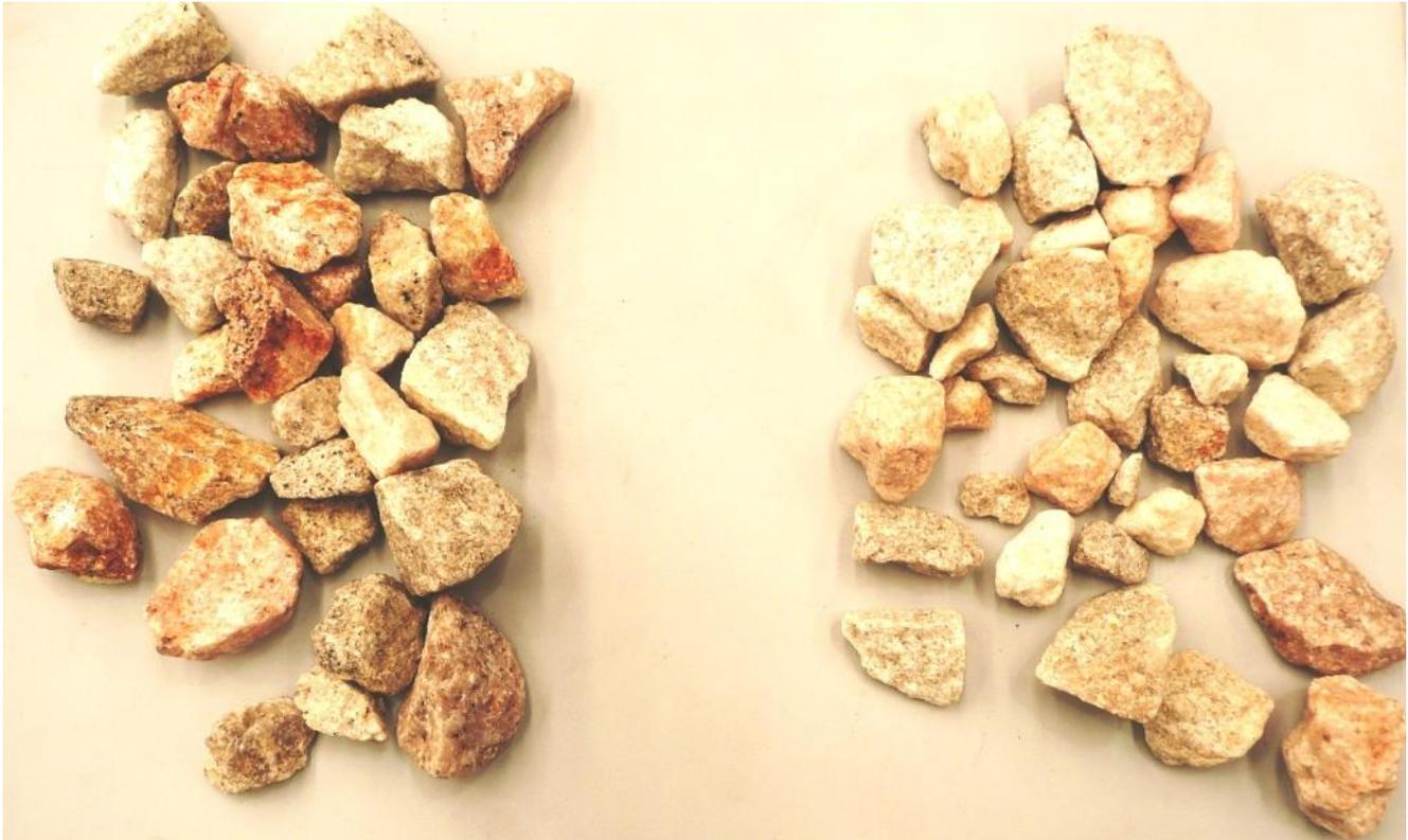
**The mineralised silexite (or product) is on the left and the unmineralised silexite (waste) on the right.**
