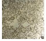
The figure to the right shows the microstructure of the first preform to exhibit extensive infiltration. These composites, which consist of interpenetrating networks of both mullite and aluminium alloy, have potential applications in friction pads for vehicular transport, impact pads for mining, and body armour for the military.
