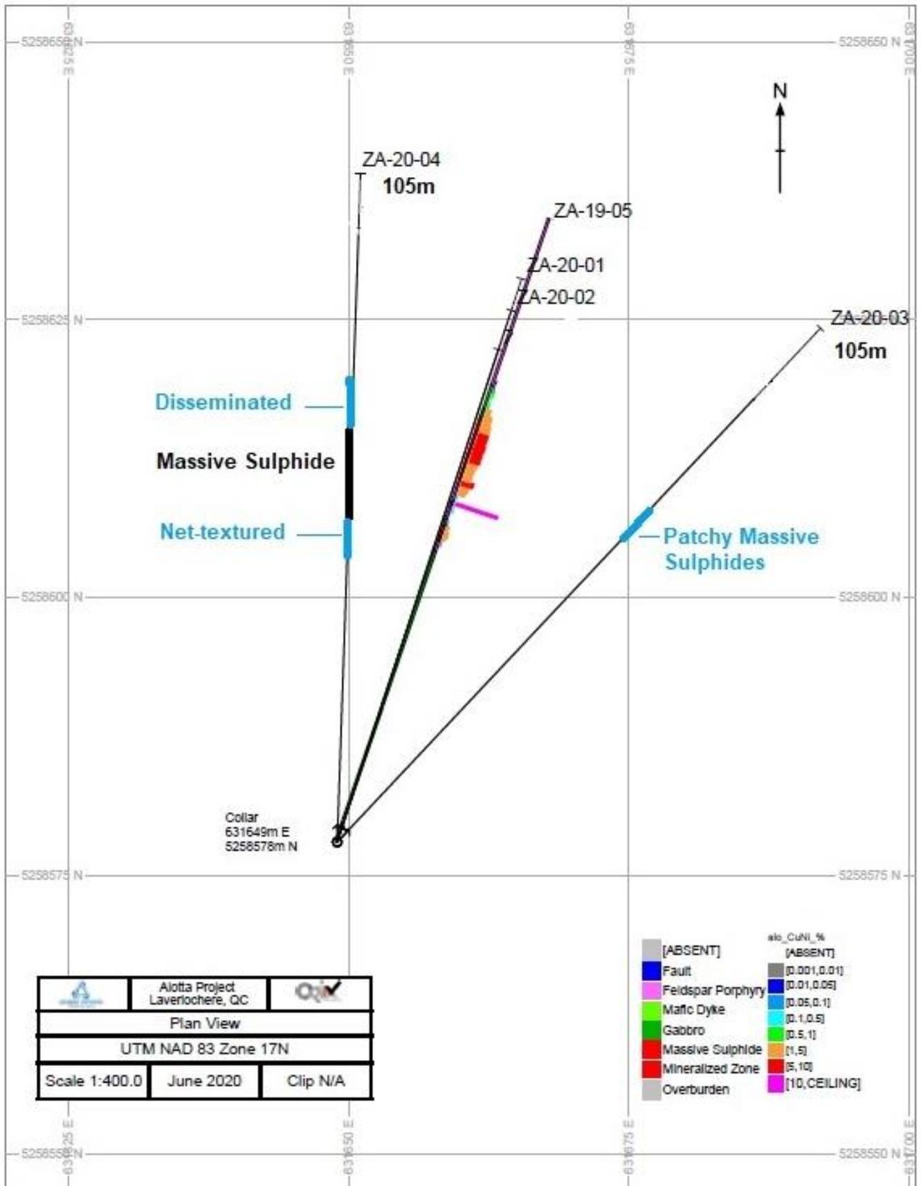
Figure 4: Plan View Hole ZA-20-03 and ZA-20-04 Intercepts
