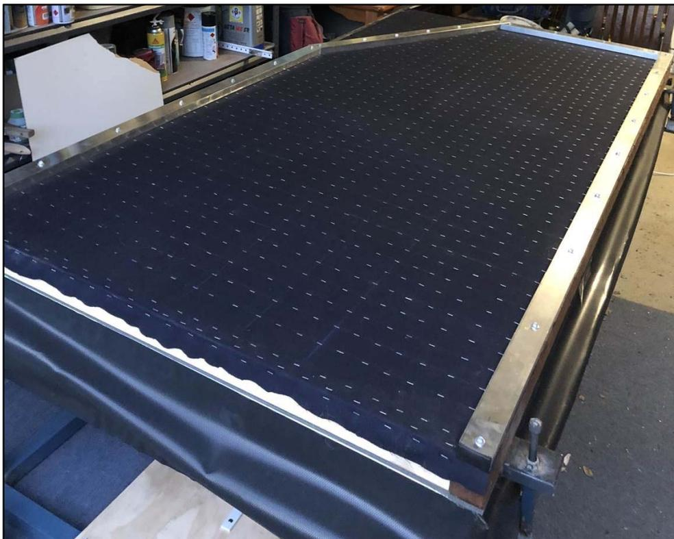
**Figure 3: Newly constructed commercial Size Air Gravity Table Testwork**
