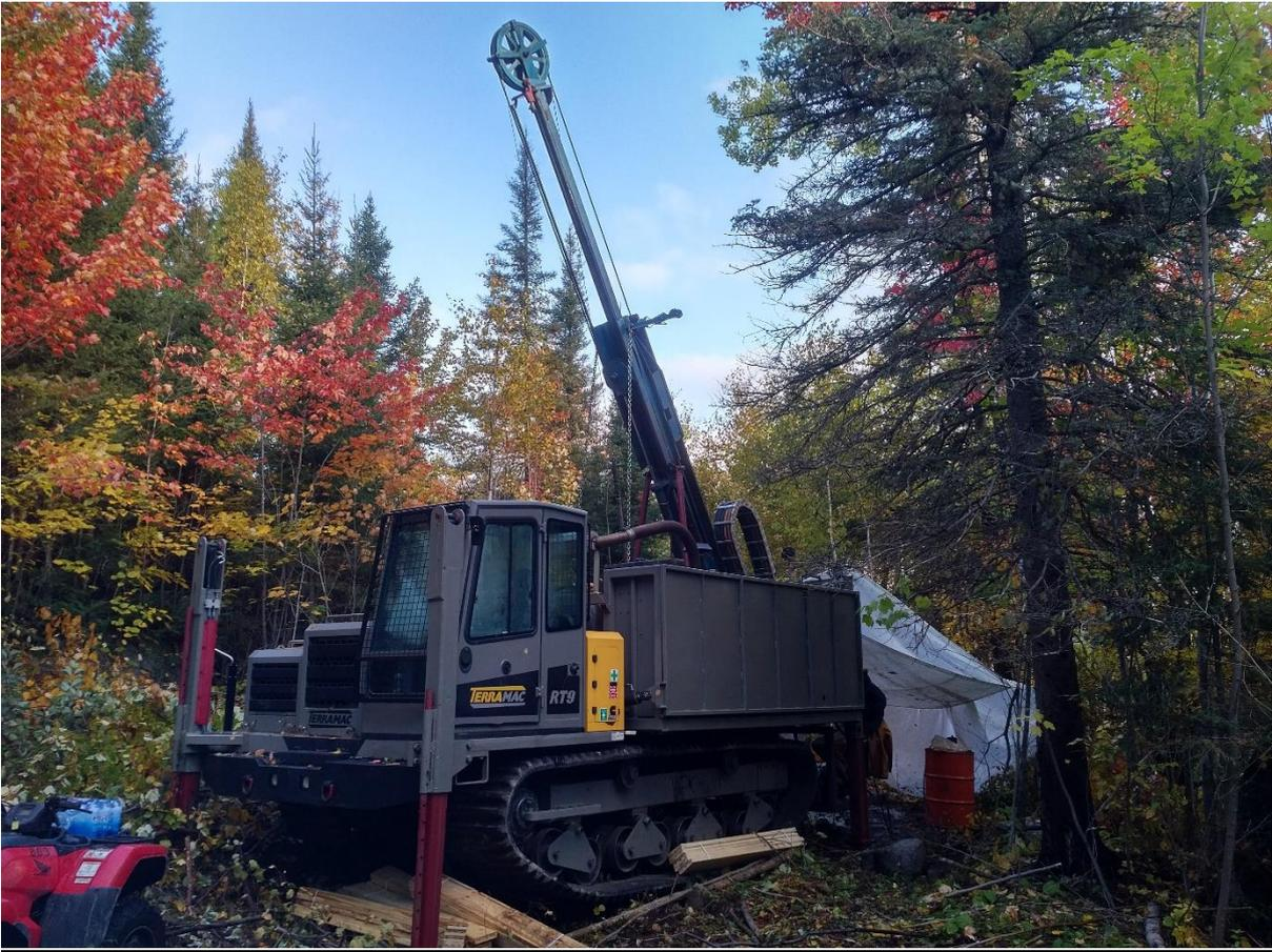
Figure 1: Diamond Drill Rig Commencing Drilling at Alotta
