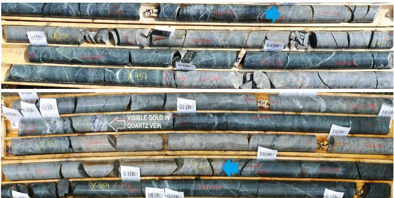
Figure 1: Very fine grained visible gold in quartz vein at ~459.8m* downhole occurs within an intermittent ~10m wide (marked by blue arrows) strong silica-carbonate alteration zone with fine grained pyrite from 453.4 to 456.1m; 457.2 to 460.1m; 461.1 to 463.1m downhole.
