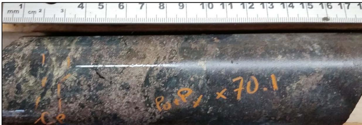
Figure 3: ZA-19-04 footwall gabbro with semi-massive and net-textured pyrrhotite + pyrite at 70m downhole
