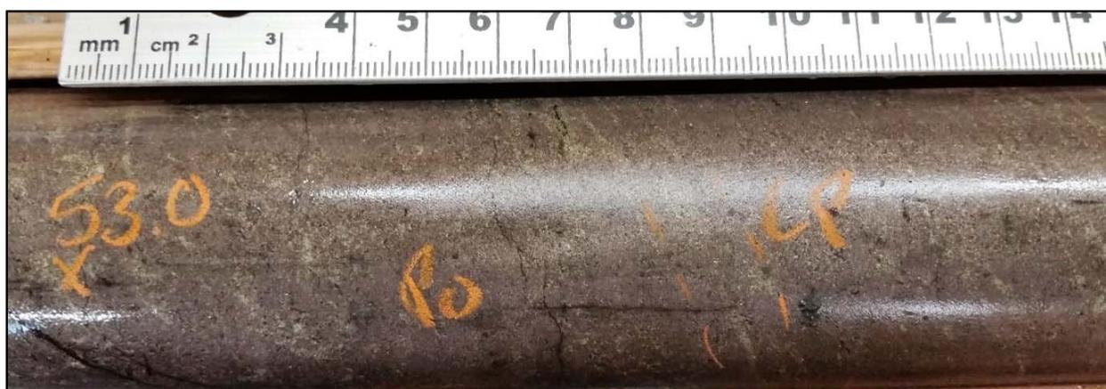
**ZA-19-04: massive sulphide comprising pyrrhotite-chalcopyrite at 53m downhole**
