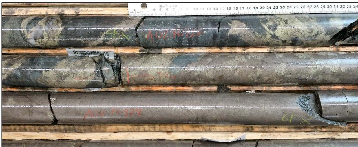
Figure 4: ZA-19-05 massive sulphide in contact with chalcopyrite mineralised brecciated feldspar porphyry at 59m downhole.
