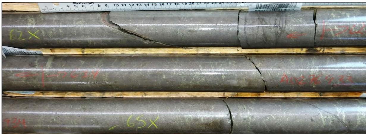
Figure 5: ZA-19-05 massive pyrrhotite with 5-10% chalcopyrite at 65m downhole.
