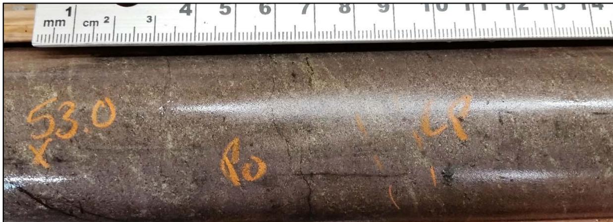
Figure 2: ZA-19-04 massive sulphide comprising pyrrhotite with bands of wispy chalcopyrite at 53m downhole.
