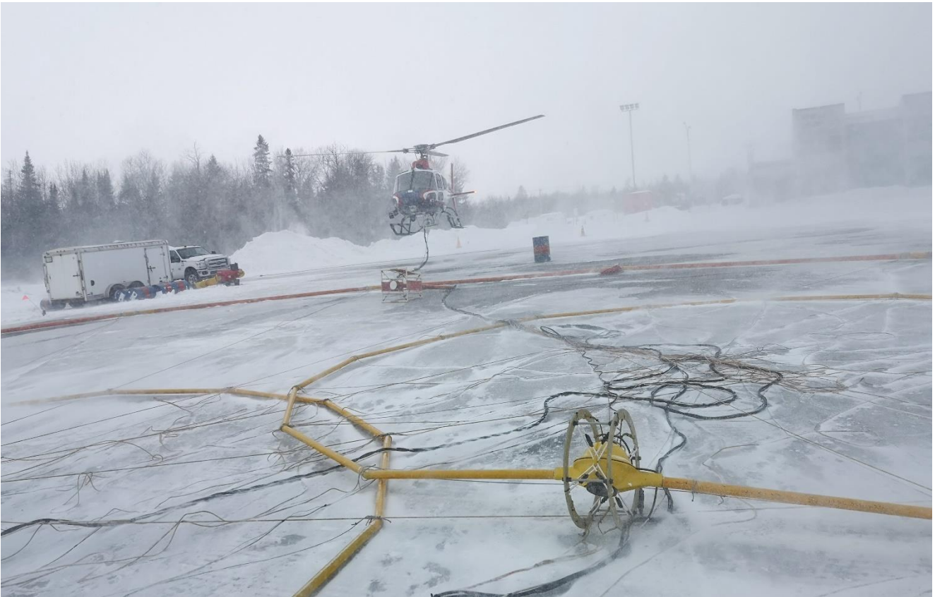
Figure 3: Geotech crew ‘landing’ the 35m diameter transmitter loop Saint Bruno Airport.
