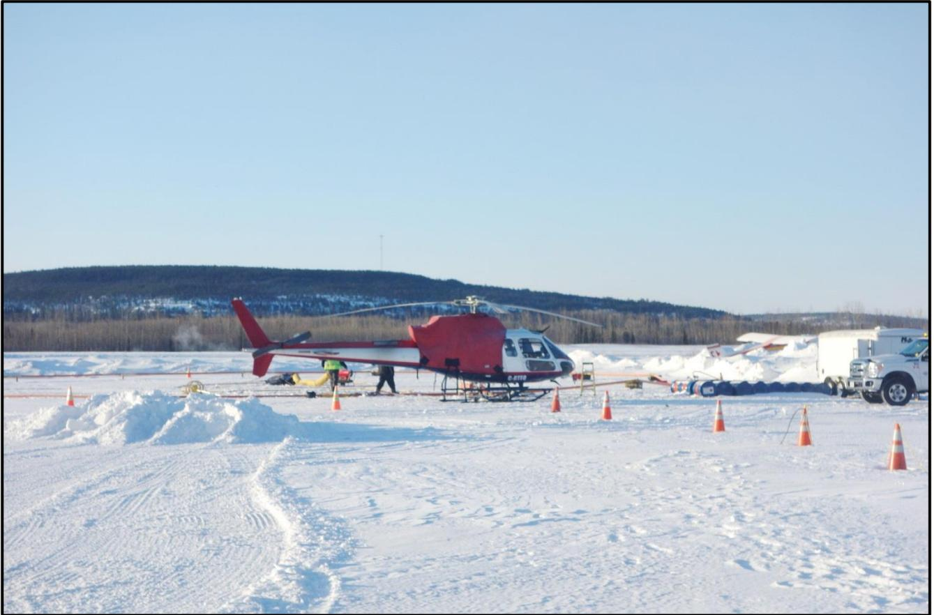
**Geotech crew preparing for take-off. The 35m diameter transmitter loop can be seen on the ground behind the helicopter.**
